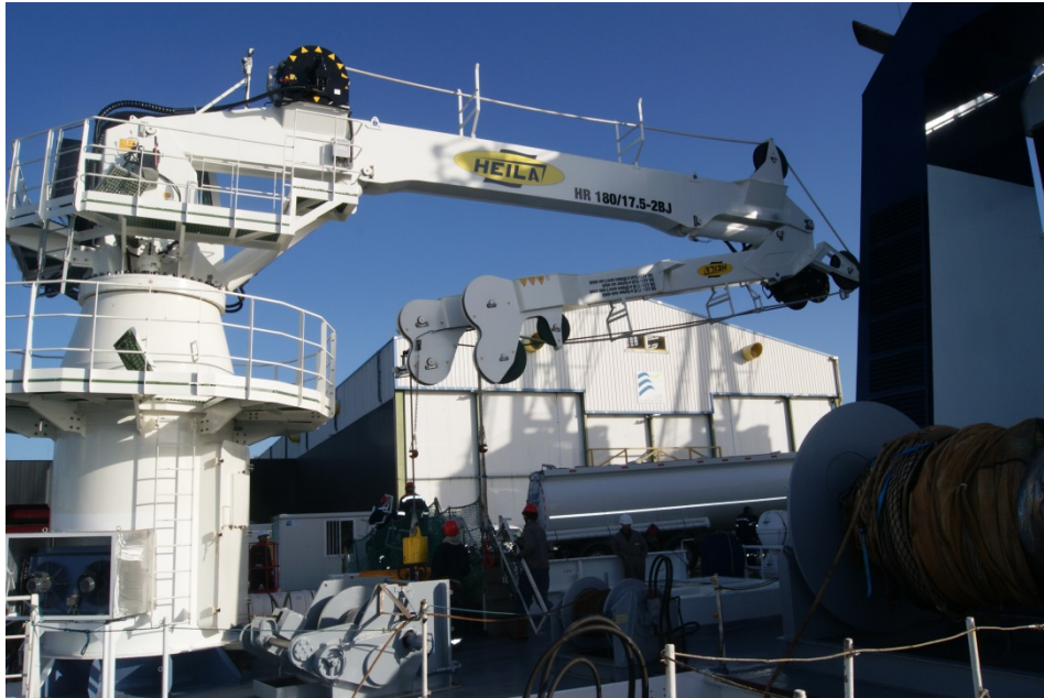
New oceanographic HEILA knuckle crane 180t.m – 2 winches (4t & 13t) – 20m at full extension
